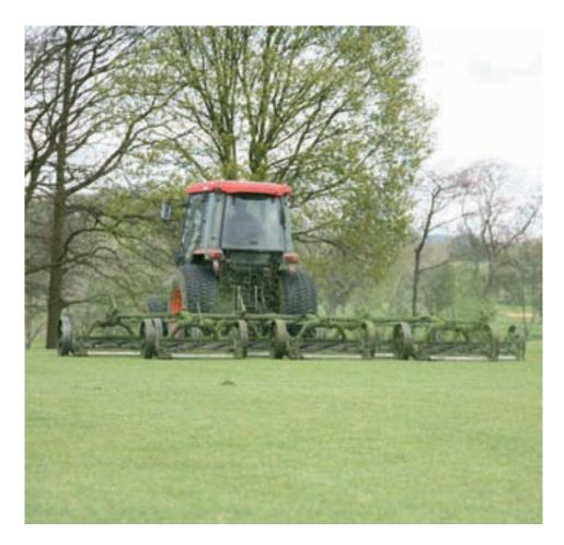
Claymore Grass Machinery is now importing the Shibaura SR525 fairway mower into the UK. It will be a tough call for the company to break into a sector dominated by the 'big three', but the new machine will certainly have its followers. Powered by a Shibaura 4-cylinder 27.9 kW (38 hp) 1,662 cc diesel, the SR525 has automatic or full time 4WD and can be specified with a choice of 7 inch reels with 7, 9 (standard) or 11 blades. As guide, the unit weights in at 1,280 kg.
