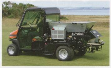
No, the Cushman Turf-Truckster is not electrically powered, but it helps define why diesel and petrol powered utility vehicles remain so popular. A well-proven golf course workhorse, it can be fitted with a range of attachments, such as a Turfco WideSpin top dresser. This sort of application is currently not as easily done with an electric vehicle, but the future may well see electric models with more power and capacity to take on this role
