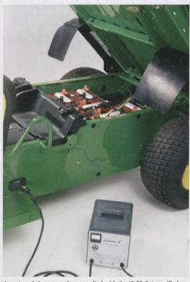
An external charger, such as supplied with the JD TE Gator, will plug into a standard single phase mains 240V ac, 60hZ wall socket. The charger senses when the charge cycle is complete and shuts down automatically. Vehicle regeneration is a common feature on modern electric vehicles, Deere suggesting the system on the TG Gator puts between three to five per cent of the full electrical charge back into the battery during a typical day's work. A single charge should last the average user a day
