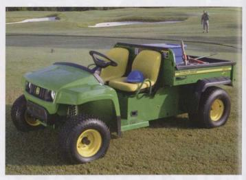
With a top speed of 15.5mph, the John Deere TE Gator should be nippy enough for most applications. It can tow up to 272kg and has a total payload capacity of 408kg. A control is fitted to slow the vehicle to a stop before changing direction. This is claimed to put less stress on the drivetrain and produce smoother operation
