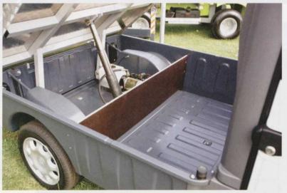
The optional Mega MultiTruck tipping body lifts to reveal a useful load area over the sealed battery compartment. Gel batteries, as opposed to conventional lead acid, are used to save space and add range. But they will be more expensive when it comes to replacing them. Payload will depend upon specification, but it is around 435kg with a tipping body
