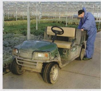
The Ransomes Jacobsen E-Z-GO MPT 1000 Electric models feature a single point battery filling system as standard. This identifies individual cells low on electrolyte and tops them up automatically. This helps reduce maintenance and equally importantly keep the batteries in tip-top condition. Also fitted with an onboard charger, the MPT 1000E can be recharged using any 13amp mains socket
