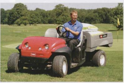
Toro, as with the other major players in the electric vehicle market, has seen steady sales of its e2050 Workman. The rear platform has a capacity of 385kg, this load being well within the machines ability over les forgiving terrain. A key to getting the best from this type of machine is to keep them charged and to not let the batteries fully discharge
