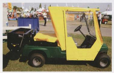
Fair enough, the style police may have something to say about the looks of a Yamaha U-MAX when fitted with a weather break style of cab. Keeping weight down, however, is critical not just for ground bearing pressures but also for battery range. When looking at electric utility vehicles, check the options on offer. It does vary between makes and models
