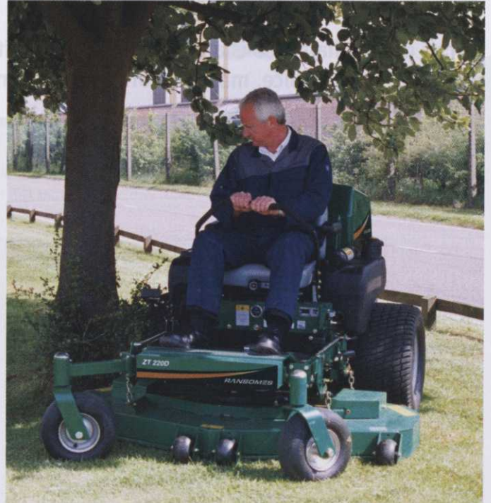
Powered by a 20hp diesel and fitted with a 60inch / 1.50m deck, the Ransomes ZT220D is claimed to have the capacity to mow up to 3.5 acres / 1.4ha in an hour. Although this will be in ideal area mowing it does serve to illustrate the serious capacity offered by zero turn mowers
