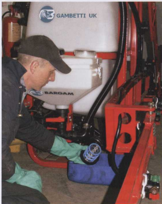
Pre-season checking of filter for cleanliness and damage
