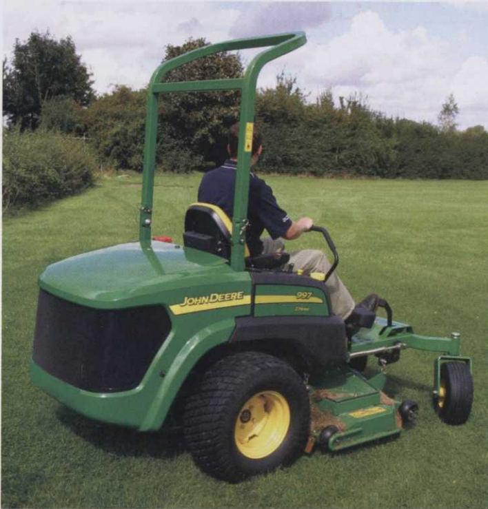
The John Deere JD 717E and JD 997 (pictured) zero-turn mowers are powered by 19hp petrol and 30hp diesel engines respectively, the larger model being designed and built in Europe and featuring a choice of side-or rear-discharge decks. Both models are fitted with folding ROPS frame and lap belt as standard
