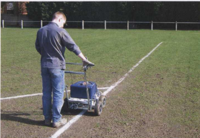
Impact Spray Line Marker showing its ability to coat both a surface with that has good grass coverage and one where all the turf has been worn away.
