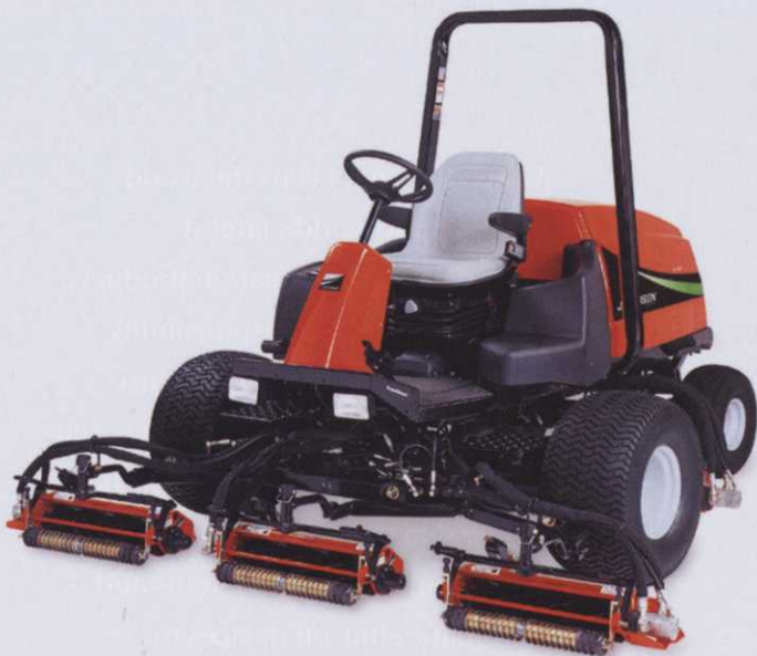
Jacobsen LF3400 and LF3800 models look pretty much the same, but offer a choice of 34 or 38hp power units to drive the five 22 inch units. The more powerful model is offered with 7 inch cylinders, against the 5 inch units on the 3400
