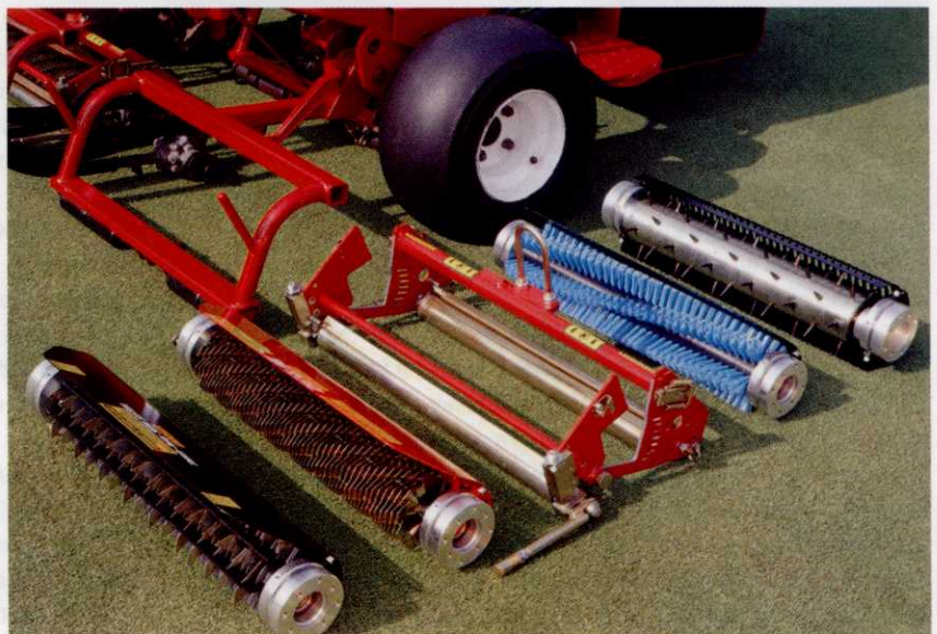
Cassette mounted equipment has opened the way for most greenscare operations to be done using a greens triple mower
