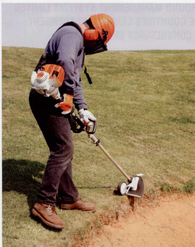
Designed predominantly as a Lawn edger, the FCB-KM unit was put to the task of trimming a bunker edge. It did a good job where the sand and grass were nearly level, but the Scrub cutter, or indeed manual edging shears, would be better for deep edges. "The jury is out on the value of this tool for bunker edging. I think it needs a bit of experience to get the best from too"
