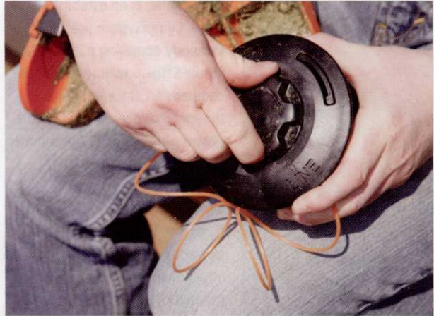
Fitting new line into the AC-KM Mowing head is an absolute doddle. Cut off a length of new line, and feed each end into the line outlets on the head. Wind in the line via the knurled base winder, cutting it either with a knife or letting the guard mounted line shear do the job for you
