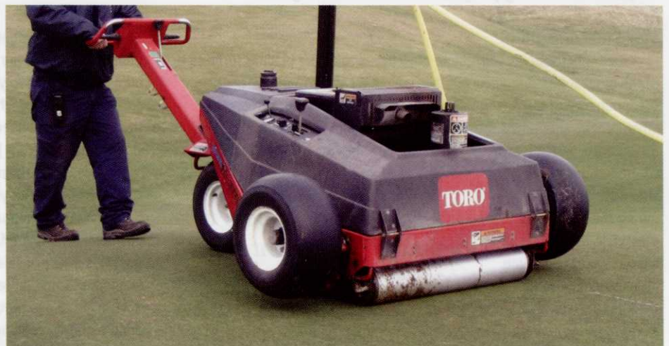
The Hydroject has the combined effect of aerating the soil and delivering water to the deeper-rooted fine grasses
