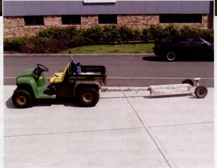
ATV towing the EMI scanner
