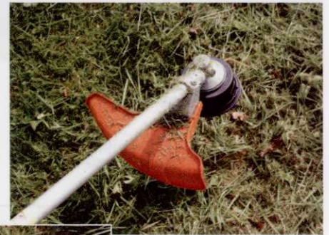
Grass cutting head, MB-KM, is the tool to select when using a brushcutter blade. STIHL offers a range of blade designs, including the twin blade pictured. In work, this left a clean cut, the cleared material appearing fair less mulched. "Normally we would use a star pattern blade, but the twin blade worked really well in long grass, leaving material that would be easier to rake up. Good guard"
