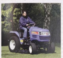
The gearbox provides six forward speeds and two reverse, ensuring the correct drive for any given application. The TM3160 also features a mid pto, ideal for driving a mowing deck and a rear pto for various mounted tools.
