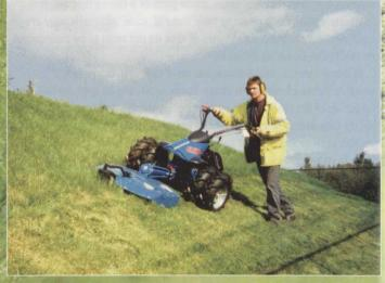
The Tracmaster Bank Commander is essentially a two-wheel tractor fitted with dual wheels and a 13hp Kohler petrol engine that can work at extreme angles without suffering oil starvation. A choice of attachments is offered, including a 1.35m cutter bar and 0.76m rotary deck. A ready to mow unit will cost from around £3,600.
