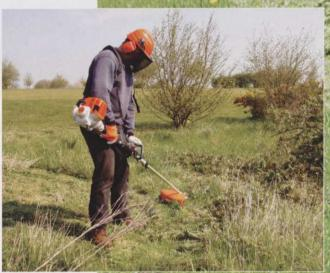
Nothing wrong with a brushcutter, but productivity over a large area is compromised and the job can be tedious and tiring, particularly in hot weather. A good harness and gloves will help reduce fatigue and vibration reaching the operator. A complete a professional kit will not leave much change out of a fator of the control of the co
