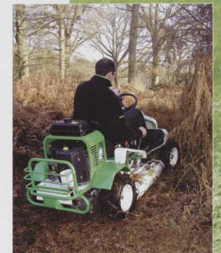
Ride-on brushcutters mix tough mowing ability with ease of operation and high productivity. As a guide, an Etesia Attila is offered in 0.85 and 0.95m versions with hydrostatic drive and chevron pattern tyres. Prices from just under £5,000 to £6,500. Tools like this can be hired for around £100 a day or £400 a week.
