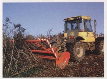
No, a heavy duty 3.0m flail scrub cutter and JCB Fastrac combination will not be a the top of the shopping list for most courses, but kit like this will make short work of areas that need clearing. It can be more cost effective to bring in a contractor to tame a really overgrown area than tackle it in-house.
