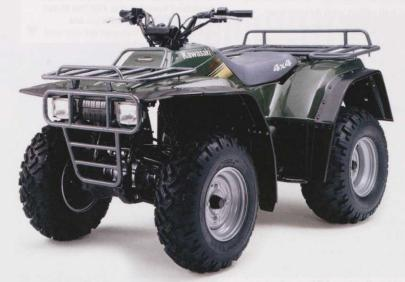
At the sober end of the utility ATV scale are machines like the Kawasaki LVF300. Available in both two and four wheel drive versions, this five speed manual model is the ideal type of working bike. Simple, easy to use and light enough to nip around on without causing damage, these models are priced from around £3,900 and will tow a decent 300kg
