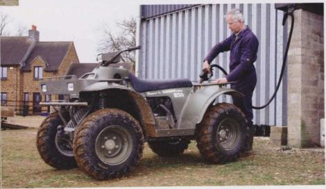
Agricultural users have long asked for a diesel powered ATV, this sector accounting for the bulk of utility bike sales. The Diesel Quads Diablo 850 answers this call, the machine having a dual range CVT automatic transmission and selectable 4WD as standard. It could well appeal to course managers looking for an economical alternative to a utility vehicle, with a price of around £6,500
