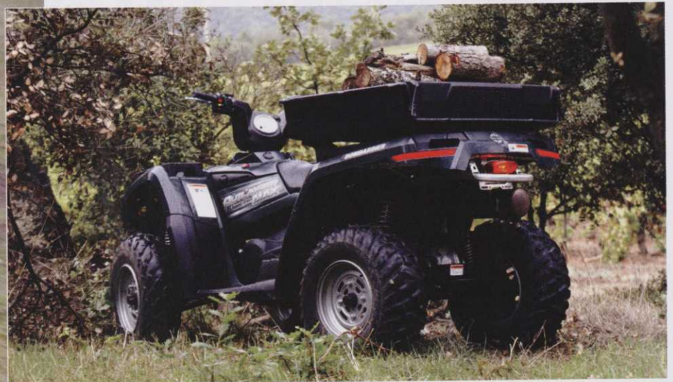
A cargo box can be fitted to a number of ATV models, but don't expect massive capacity or dimensions. The Can-Am Outlander Max will only carry around 95kg, its high load height also working against it. But fit a trailer as well, and the package starts to make more sense. A 650 Outlander, which is a really powerful ATV with easily enough torque to handle a capacity load, will cost from £6,800
