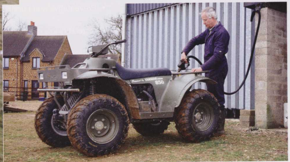
Agricultural users have long asked for a diesel powered ATV, this sector accounting for the bulk of utility bike sales. The Diesel Quads Diablo 850 answers this call, the machine having a dual range CVT automatic transmission and selectable 4WD as standard. It could well appeal to course managers looking for an economical alternative to a utility vehicle, with a price of around £6,500
