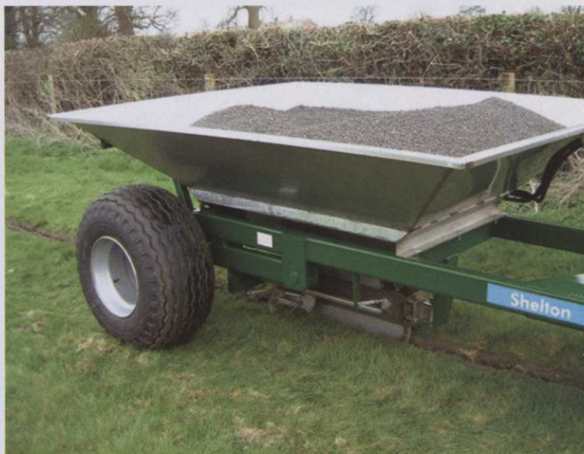
Fastflow 3 tonne capacity gravel backfiller places permeable fills at fast walking pace; no spills, no wastage
