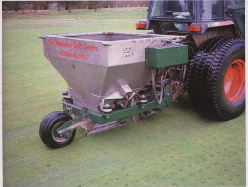
Gravel Band Drainage - equally effective on a green as on a fairway
