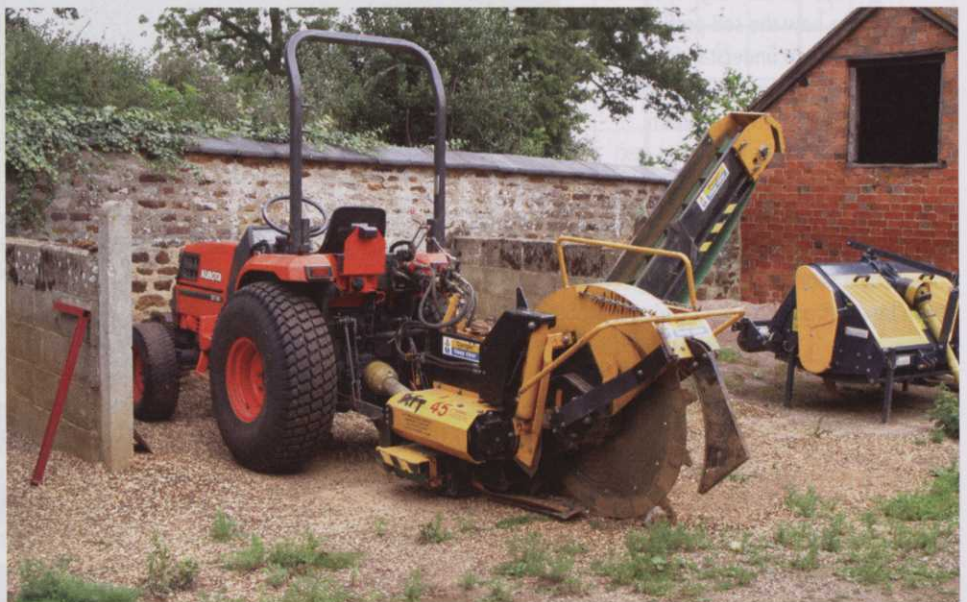
Ian Marshall, Head Greenkeeper at Wellingborough Golf Club, has carried out in house drainage and irrigation pipe installation on the course at Harrowden Hall using an AF Trencher, AF45, fitted with a Slitting Wheel. A job quoted out at £50,000 was carried out using the pictured combination for around £15,000.
