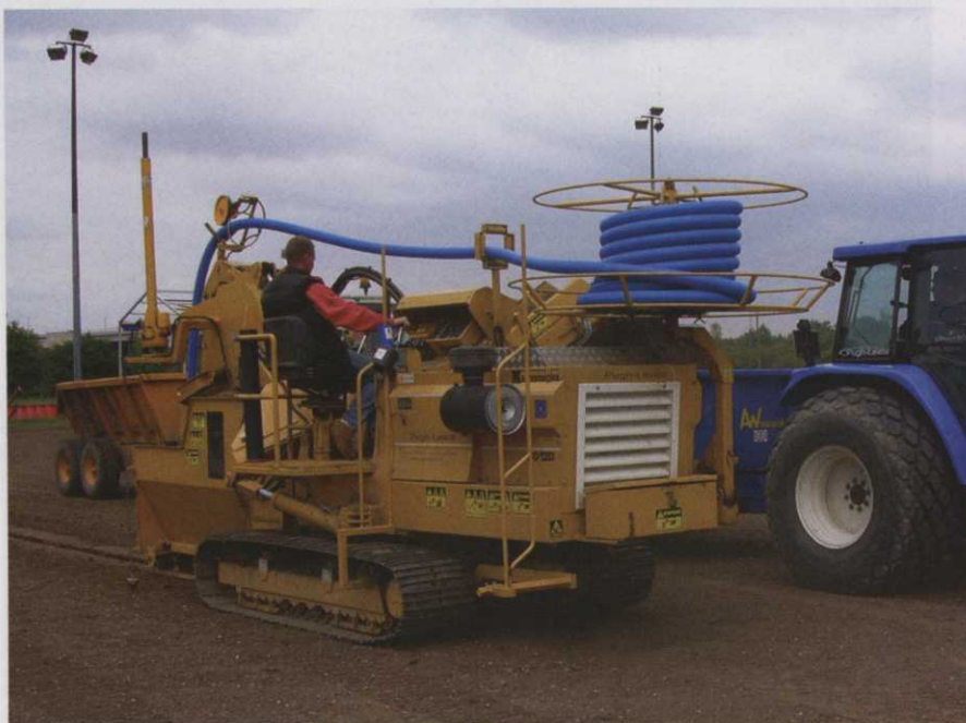
25mm land drainage pipes fits into a trench narrower than a golf ball
