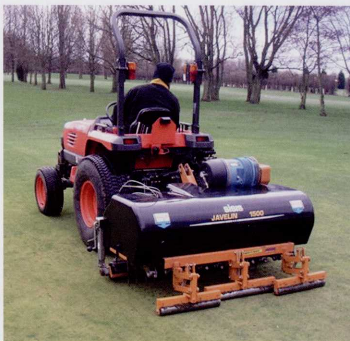
The Sisis Aer-Aid System in action relieves compaction, improves infiltration rates and combats Black Layer, claim the company
