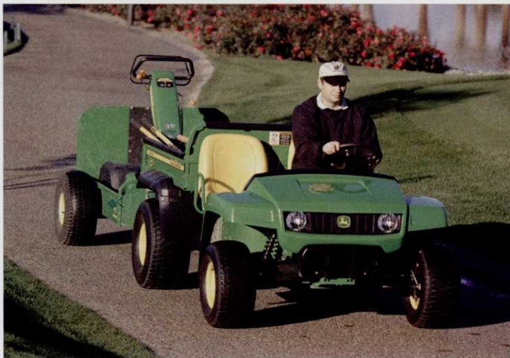
Latest Deere 'T' series Gators benefit from more power and better brakes; fuller details unavailable at the time of going to press. Note the use of a low loading trailer. This makes it far easier to load and transport heavy items of kit such as pedestrian greens mowers
