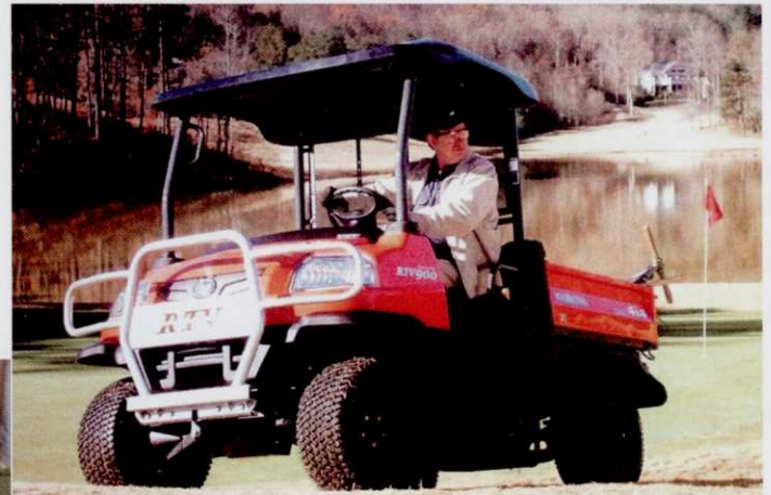
Kubota are alone in offering a sophisticated hydrostatic drive system on its recently introduced RTV900. Hydrostatics have a great deal to offer, and are well proven, the system offering the potential to potter along at a reduced engine speed. This is something a CVT automatic struggles to manage
