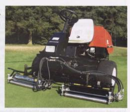
the range of TurfWorks cassettes are British designed and manufactured using Sheffield Stainless Steel. The manufacturing process utilises integrated laser cutting by means of ferrous and non-ferrous materials to an accuracy of 0.1mm. A broad range of advanced engineering equipment, including the latest and most advanced CNC milling and turning machines, are used on items such as bearing housings and drive couplers.
