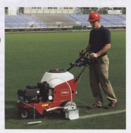
stops. Its new Express Clean System incorporates an onboard fresh water tank that cleans the line and nozzle at the flick of a switch. So the operator can take a break whenever they want without the line painter clogging up.
