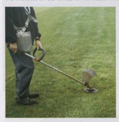
New to the UK, Powerhead is a high speed cutting attachment, designed to shave hours from the tedious job of trimming around sprinkler heads.
