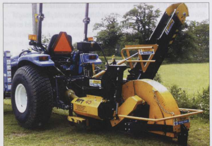
▲ Cutting wheel for neat narrow trenching
