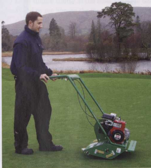
Sean Reilly, Loch Lomond Golf Club, tackles compaction with a S500 pedestrian aerator manufactured by Dennis of Derby
