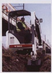
hydraulic clamp attachment. Equipped with cab and rubber tracks, the 323 has an operating weight of 1743 kg. Maximum reach at ground level is 4014 while maximum digging depth is 2297 mm.
