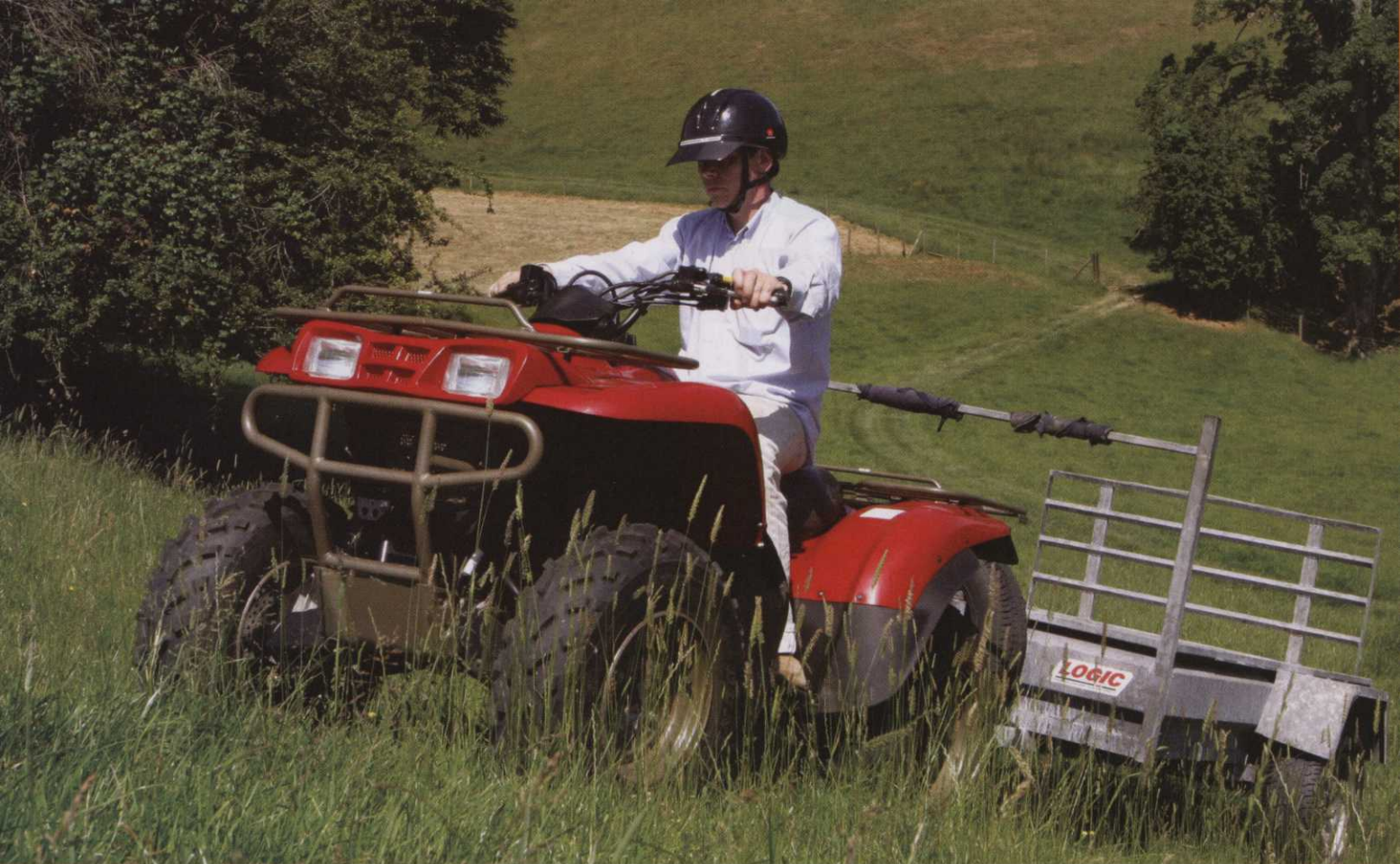
Hang a trailer onto the rear of an ATV, and it is immediately more useful. A two-wheel drive ATV is fine in easy going, but if there is steep terrain in the job mix, go for 4WD
