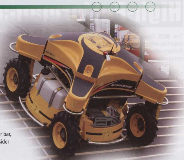
▲ Remote controlled mowing comes of age with the Ransomes Spider. Designed to operate on slopes of up to 40 degrees, the machine has a light footprint as it has no operator and related controls. Remote technology at present is costly, but this type of equipment may become more affordable if the concept takes off.
