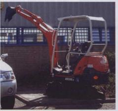
speed of 2.2km/hr. Its 950mm long arm provides a maximum digging force of 7.2kN (735 kgf) and the digging force of the bucket is 13.0kN (1327 kgf).
