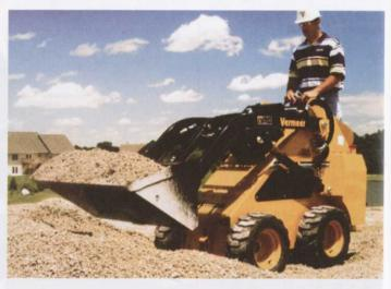
S600 has excellent mounting plate visibility, boom and tilt lockout, operator presence including auxiliary hydraulics, neutral start interlocks, built-in lift-hook and tie-down locations and a parking brake.
