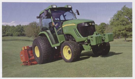
The horse power of the five models range from 31hp to 52hp, and the lower emissions engine features up to 30 percent more torque and lower fuel consumption, which all combine to provide an improved performance.
