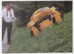
There are significant health and safety benefits to the operator. It is no longer necessary to stand with a string trimmer or walk with a mower on steep slopes putting excess pressure on hip, knee and ankle joints which can lead to joint stress in later life.
