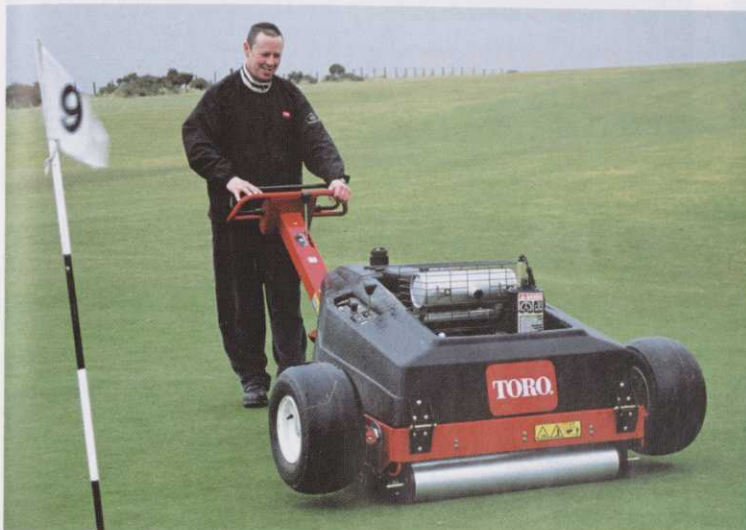
▲ The Toro HydroJet water-injection aerator is ideal for summer aeration with minimal surface disruption.
