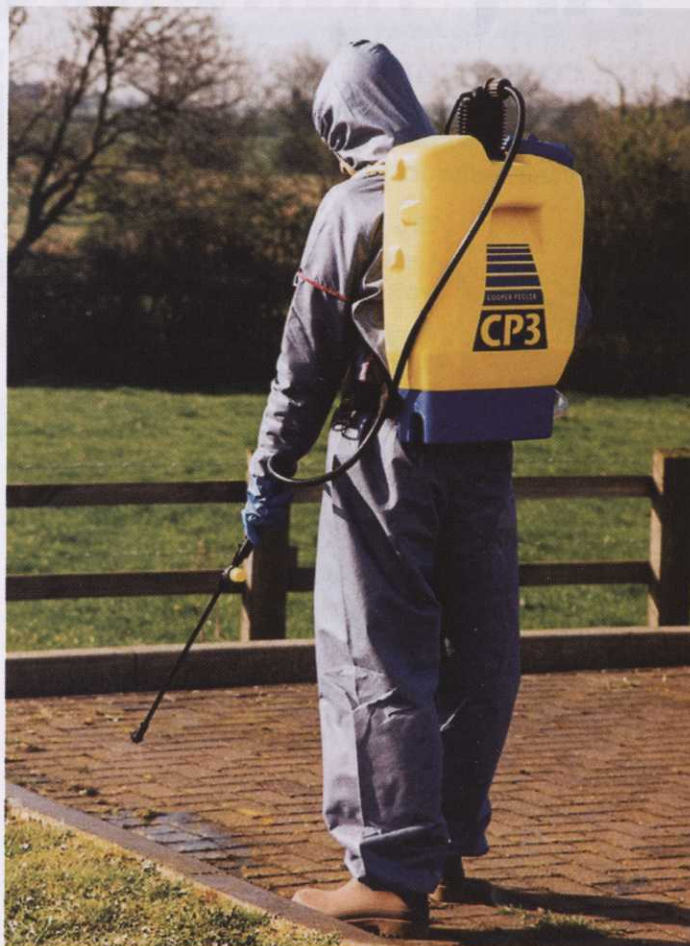
▲ Flood jets are commonly used on knapsack sprayers as they provide a wide swath and are less prone to nozzle blockages
