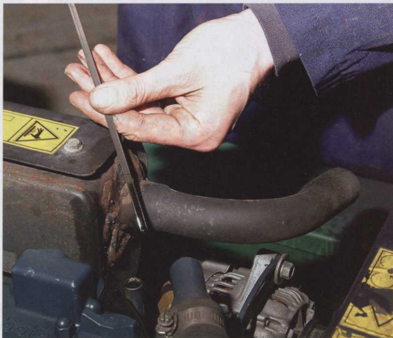
▲ Every time a machine is used ensure the engine oil level is correct
