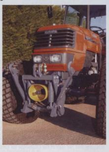
The front pto gearbox is capable of delivering up to 200 hp, and hence is well on top of the job with even the ME9000. It features an oil immersed multiple plate clutch using electro hydraulic "Soft Start" engagement to avoid "snatching" and possible implement damage when the pto is engaged.
