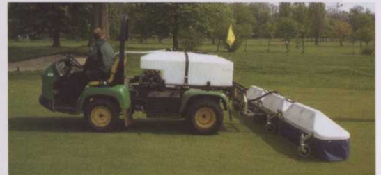
▲ JD series 600 ltr sprayer and 4.5m Hurricane on a ProGator at Roehampton
