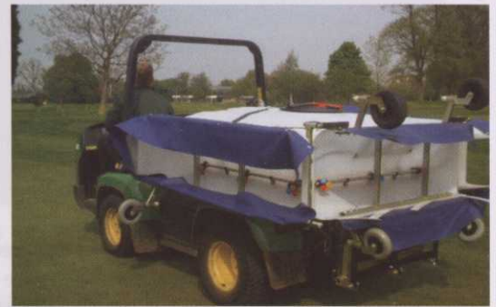
▲ JD600 with 4.5m Hurricane neatly stowed around the tank for transit
