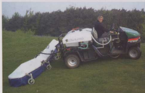
▲ RJ series 600 ltr sprayer and 4.5m Hurricane on a Cushman at Pedham Place, Kent
