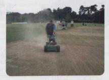
wheels are independently controlled, this gives a turning radius of ZERO giving the operator full control for manoeuvring in any situation. There are 2 cutting widths available, 62" and 72" with an option of side or rear discharge.
