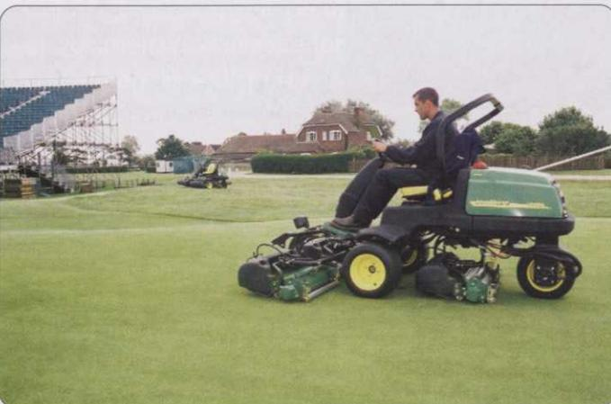
The most important areas are the cutting units and the system that operates them. The efficiency of hydraulics depends on a constant pressurised oil flow, so if a single pump has to operate a number of facilities then the mower's efficiency might be reduced. Triples that have hydraulic systems specifically dedicated for lift, power steering and cylinder and wheel motors are features worth taking into account.
