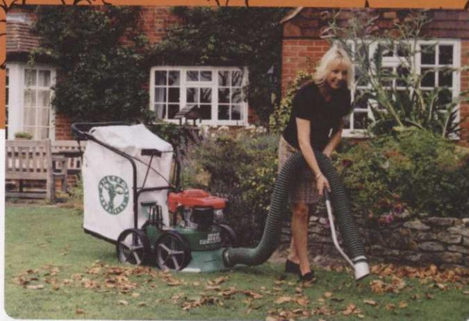
powered blowers are also available, these blow the leaves into windrows ready for collections. This then means that large amounts of material is accumulated in one place so some form of loader will be required. This can be in the form of a towed unit or one that fits to the tail board of a trailer, skip or vehicle buck. They are basically a vacuum unit with a large diameter inlet hose and adjustable outlet chute.
