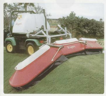
Windfall's enclosed booms give less drift in a 24 mph wind than a conventional open boom in a 6 mph wind, allowing grounds professionals to maintain work schedules in less than ideal conditions. The aerofoils have front and back mounts to secure them even during high speed transport.
