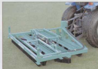
The Multi-Brush instantly transforms into a 6' wide zig-zag brush for greens
