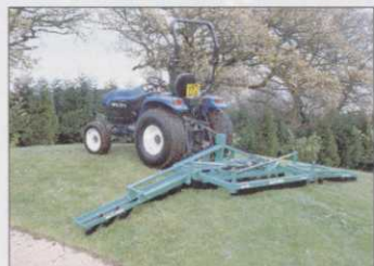
Three individual brush heads follow the contours of fairways and around your bunkers
