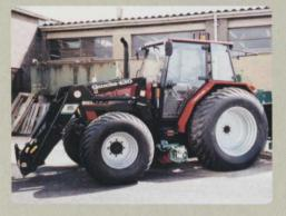
distributed, but this is only part of the picture. The tread pattern is also important in reducing slippage and increasing the machine's efficiency. Stability is another factor, especially on uneven or sloping terrain. With the right tyres fitted it is possible to work on soft, wet areas, with minimal marking or damage to the grass.
