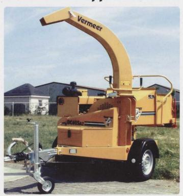
ing and better stability. A wide axle with wheels mounted outside the chassis, enables the infeed table to be mounted 10 cm lower than its predecessor. This new stable, low design, not only makes it easy to get the
