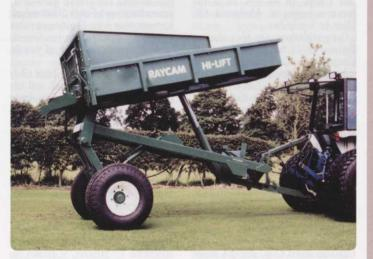
low ground pressure tyres to eliminate the risk of turf damage, even when fully loaded.
