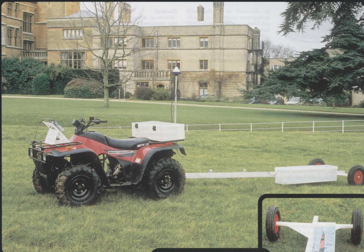
The surveys can be done by hand held equipment or, as above, with a quad bike trailing the sensors
