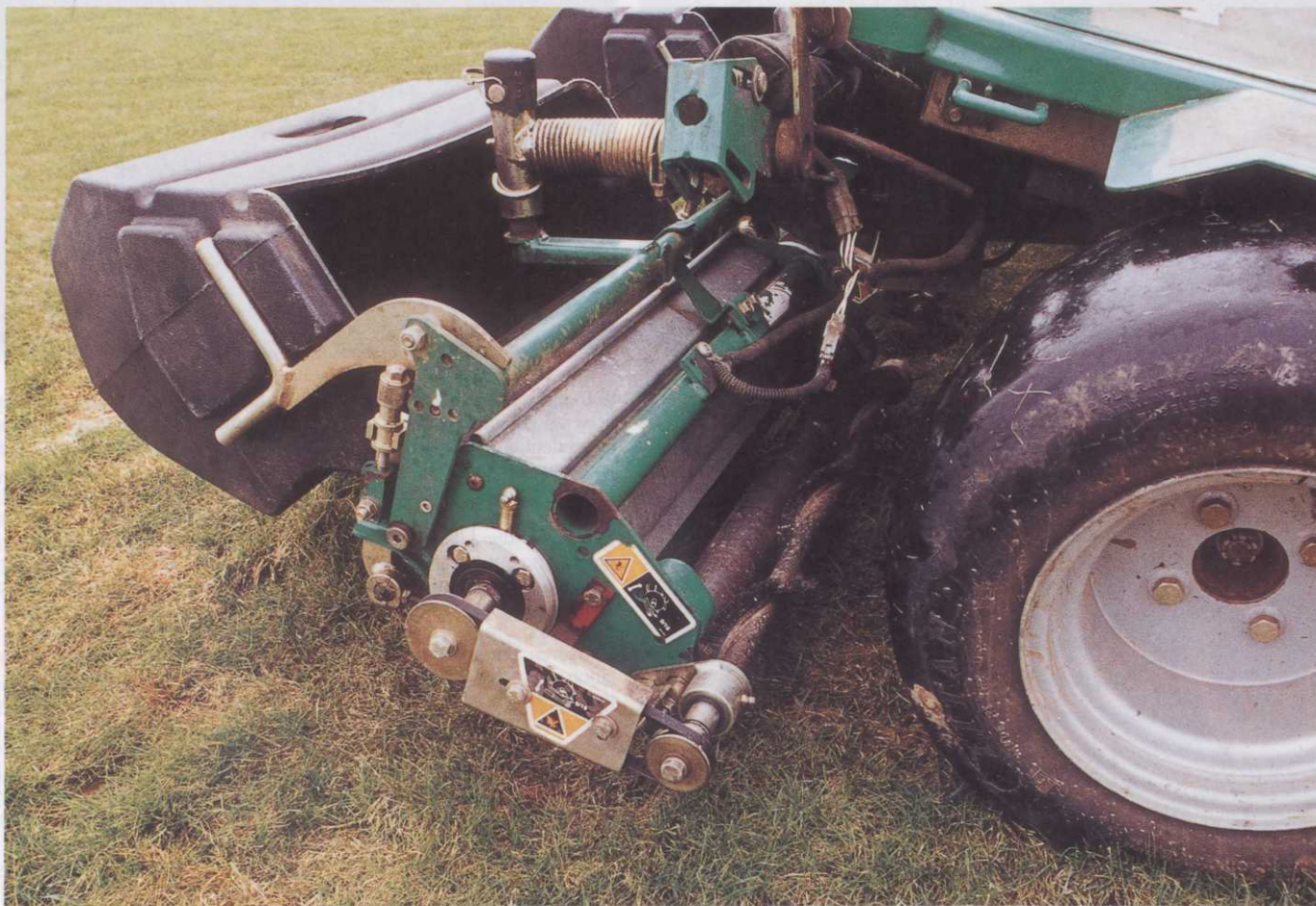
Above: The bearings of the powered roller brushes are packed with a special lubricant to reduce friction
