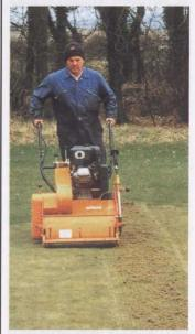
It incorporates the SISIS Rotorake contra-rotation principle, whereby the reel rotates at high speed against the direction of travel. The blades therefore cut upwards continuously throwing fibre forwards rather than pushing it into the surface. The machine is also held to the ground to maintain a regular working depth.
