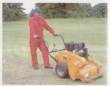
It also contributes to aeration. The clean, continuous slits assist water and air absorption through a heavy thatch layer, and integration of top
