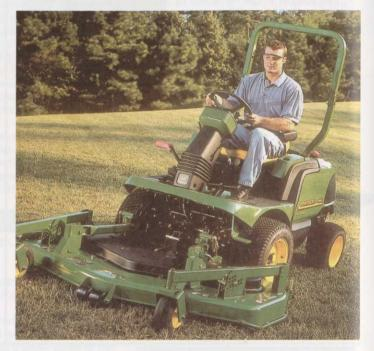
transfer and cruise control, a rear hitch and hard or soft cabs; heavy duty attachments include a 1.19m snow blower, 1.37m front blade and 1.52m rotary broom.
