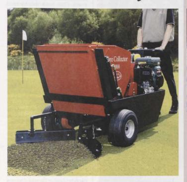
The CC20 and CC30 share key features that set them apart from other machines. Both incorporate a specially designed 'floating' rotary impeller collection head that adjusts itself automatically to suit the prevailing ground conditions and does away with lengthy set-up procedures. The impeller throws the cores into the collection hopper at such speed that they shatter, meaning that no space is wasted and that the maximum volume of material is gathered before emptying is required.
