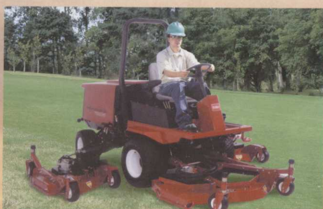
GROUNDMASTER 4000-D Big, powerful and durable, Toro's 4000-D Groundsmaster won't let you down. Its 56hp engine combines with three decks to give a maximum cutting width of 11ft for great productivity over the toughest terrain.
