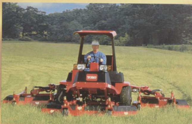
GROUNDMASTER 580-D With a massive 80hp engine and covering a huge 16 feet cutting width with its three decks, the Groundsmaster 580-D is a force to be reckoned with yet still delivers manoeuvrability, traction and stability over rough ground.
