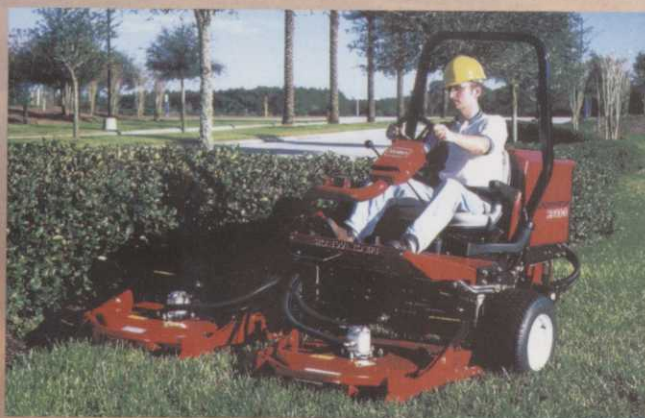
GROUNDMASTER 3500-D SIDEWINDER Toro's unique Sidewinder rotary mower, with its innovative ability to shift the cutting units to the right or left, gives a quality finish right up to the bunker or water's edge. With a 35hp water cooled engine and three 27in floating rotary decks, its productivity is superb.
