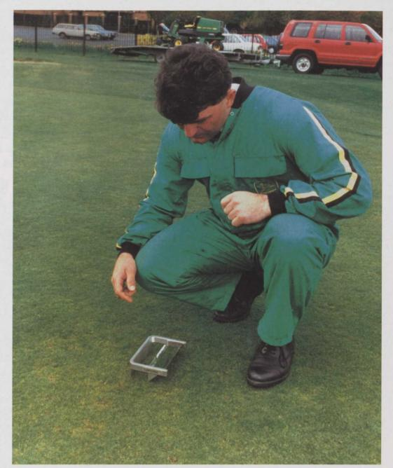
seen examples of a pedestrian mower set at a height of cut of 3 mm but using a prism gauge we find that the sward is left at 2 mm. These differences may seem very small, after all we're only talking about a millimetre or so aren't we?
