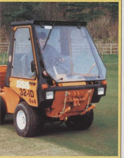
avoids surface marking when turning. A patented weight transference system on the rear three-point-linkage applies extra pressure to attachments when required, thus eliminating the need for extra weights. Low ground pressure tyres are standard. Power steering combined with a pivot steer chassis gives a tight turning radius on headlands and around obstacles.
