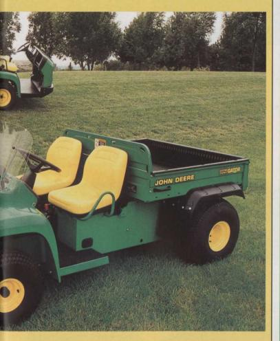
of either two or four wheel drive. The cargo box has hydraulic lift and can take loads up to a estimated 875kg. When not needed the box can be quickly removed. The company has also introduced a top dresser attachment with a .54m capacity and a spreading width of 1.47 metres. This unit is run off the vehicle's hydraulic system.
