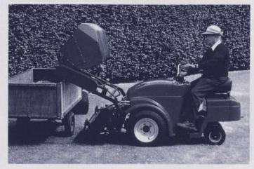
incorporated, including the use of a rear Slick tyred roller wheel to provide full width rolling and prevent rutting on soft ground. Also the ability to swing the mulching mower to either side, whilst mowing to avoid trees and shrubs. Frank Moore says "When I set out to
