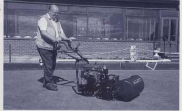
rollers and available as a 20" or 24" machine it will provide excellent stripping on lawns, pitches and any other area of fine turf.
