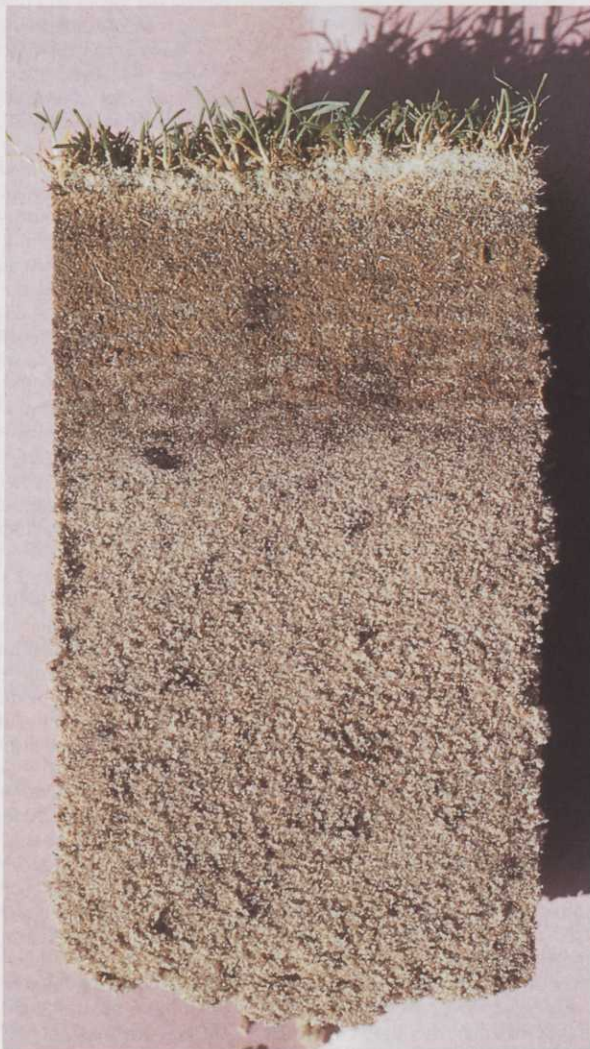
Above: A core sample taken from a predominately sand based green, which over the last five years, has received little thatch management
